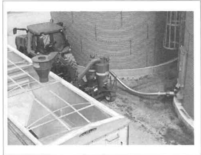
Fig. 4-11 Bin Clearance 12ft (4 M)
