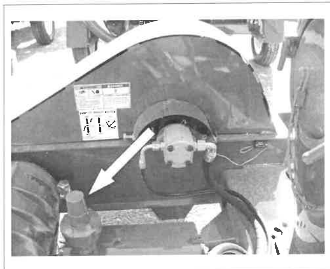
Fig. 5-33 Pressure Relief Valve.
