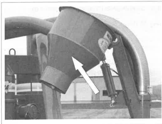
Fig. 5-6 Check the Wearliner in Discharge Cyclone.
