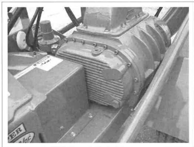
Fig. 5-4 Blower Reservoirs (Front)
